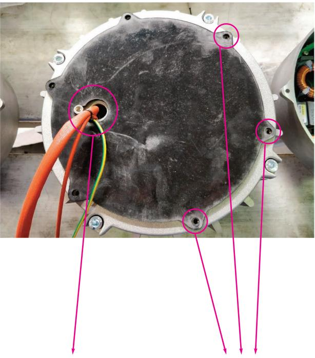
Position the motor part so that the motor cables are toward the left.
