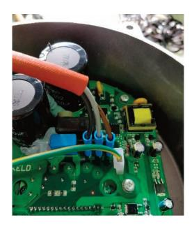
Insert the faston connectors on the motor phase electronics according to the following diagram:
