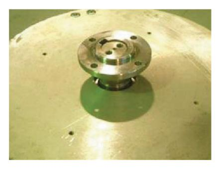
Slide off the fall protection plates and remove the hub from the shaft
