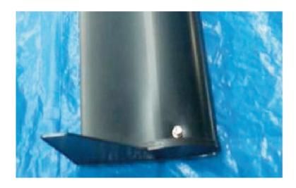
Unscrew the screw holding the plastic Winglet to the blade
