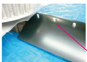
TOP PART OF THE BLADE FIXED WITH THE SELF-LOCKING NUTS
