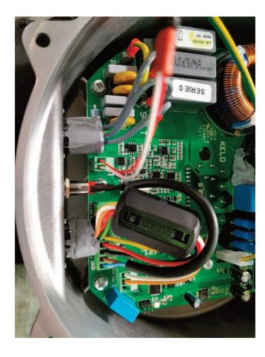
Insert the motor temperature sensor green connector, with White/Red wires, in the corresponding connector on the electronics (positioned as shown in the figure).
