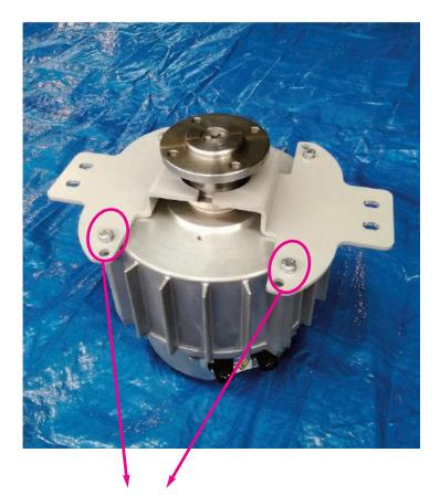
Remove the screws fixing the fall protection plate to the motor
