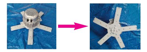
Before starting, overturn inverter motor so that the blade fixing starwheel is on the upper side
