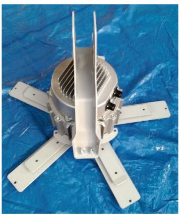
After having set the inverter motor on the ground, remove the bracket fixing screws.
